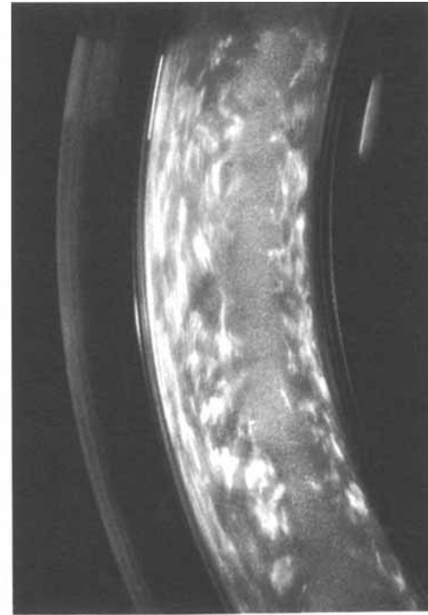
FIGURE 19. Sequence of flow visualization photographs showing the development of the flow instabilities during the spin-up process at C = 7540 . The elapsed times after the start of the container are (a) 0.5 s, (b) 0.75 s, (c) 1.0 s, and (d) 1.25 s.
