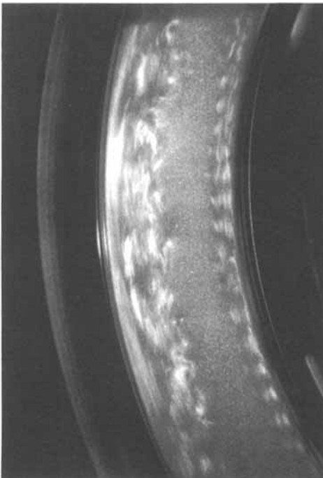
FIGURE 19. Sequence of flow visualization photographs showing the development of the flow instabilities during the spin-up process at C = 7540 . The elapsed times after the start of the container are (a) 0.5 s, (b) 0.75 s, (c) 1.0 s, and (d) 1.25 s.
